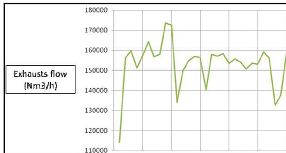
Due to the high sulphur content, it is not possible to cool the exhausts below 110°C. Thus, the potential recoverable thermal energy is around 2,5MW<sup>6</sup>.
