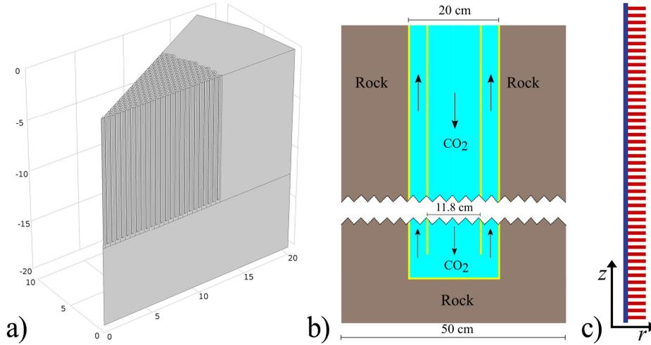
Figure 1: a) Drawing of a 30° sector of the ground heat storage, b) sketch of a single coaxial exchanger, c) 1D/2D computational model (deformed in the radial direction) - fluid domain (blue) and rock domains (red)
