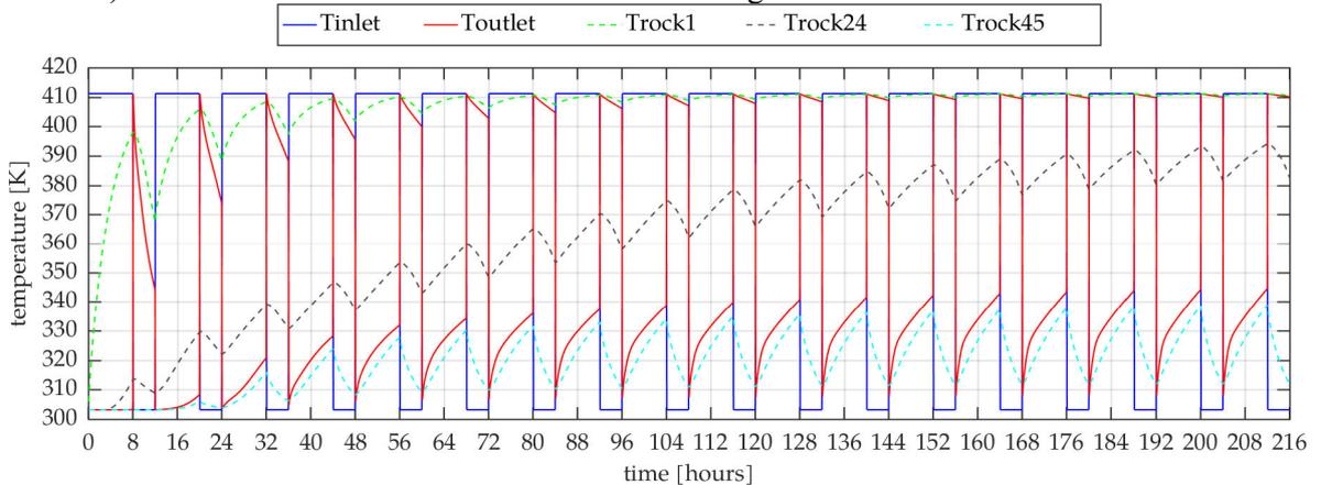
Figure 2: Temporal evolution of inlet and outlet temperature for a series of exchangers (continuous lines) and volume-averaged rock temperature for 1<sup>st</sup>, 24<sup>th</sup> and 45<sup>th</sup> exchanger (dashed lines)
