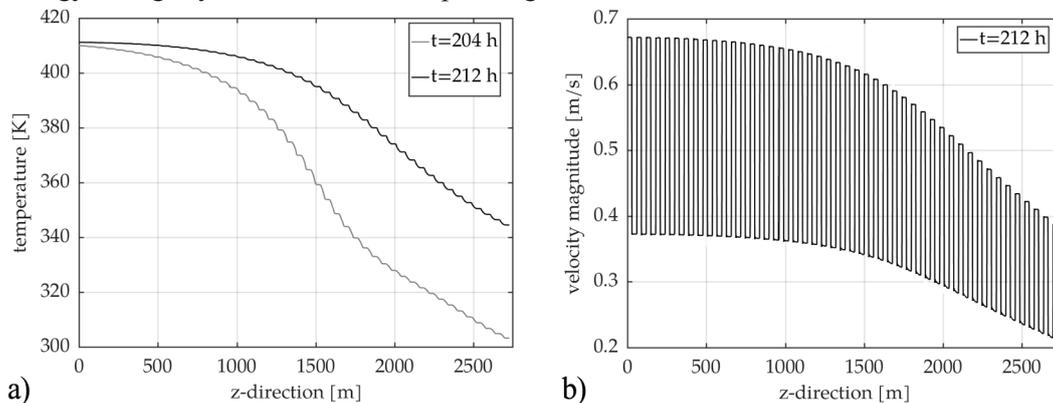
Figure 3: Spatial distribution of CO<sub>2</sub> temperature (a) and velocity (b) along a series of exchangers during charge (212 h, end of last charge) and discharge (204 h, end of second-last discharge)
