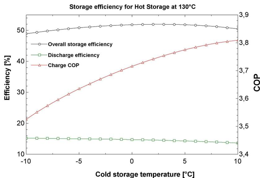
Fig. 6. Storage efficiency as a function of cold storage temperature ( $(T_{\text{hot}})_{\max} = 130^{\circ}\text{C}$ ,  $\Delta T_{\min} = 1\text{K}$ ).
