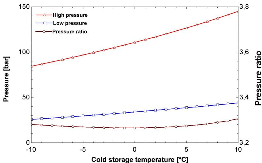
Fig. 8. Pressures of the system as a function of cold storage temperature ( $(T_{hot})_{max} = 130^{\circ}C$ ,  $\Delta T_{min} = 1K$ ).
