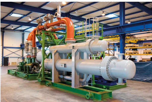
3500 kWe ORC – BaoSteel plant, Shanghai, China
