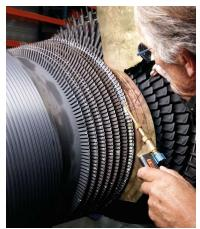
Interventions on smaller turbines are performed in Enertime's workshop in the Vendée, where the company also designs, manufactures and maintains it own turbomachinery on daily basis.
