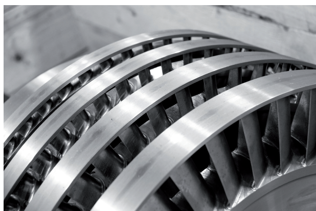
Enertime axial multistage turbine
